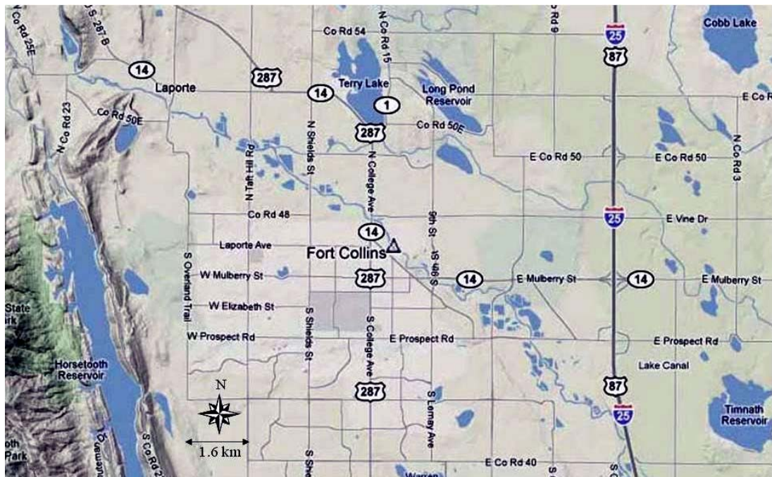
Figure 1. The Cache la Poudre River in the vicinity of Fort Collins, Colorado, USA. The triangle shows the USGS gage on the Poudre River at Fort Collins. The map also shows the many water-filled gravel pits along the river, many storage reservoirs, and a major canal diverting water downstream of the river's Taft Hill Road crossing.
